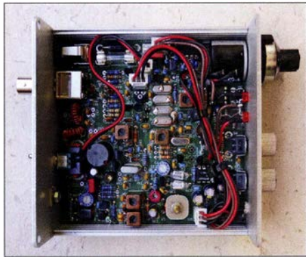
40-m-CW-Transceiver BTR18 Fotos: DK3RED
